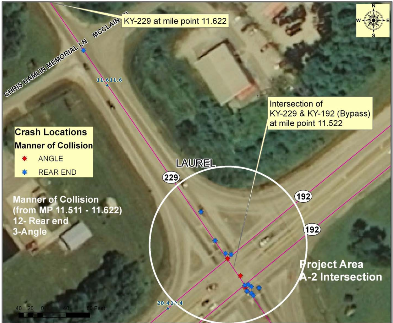
Figure III-16: Section 3- KY-229 High CRF Collision Location (from MP 11.511 to MP 11.622)
